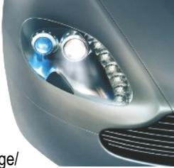
conventional halogen for main beam. While we have to agree that Xenon's are most useful on dip, where they reduce dazzle from other car lights and improve visibility when there is oncoming traffic, we would have expected a Bi-Xenon system to match the car's performance potential. Aston have responded to this, with powerful Bi-Xenons first introduced on the Rapide and now standard on Virage, Vanquish and 2013MY DB9.
